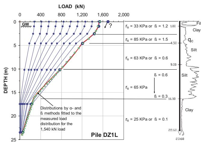
effective stress calculations back-calculated to fit the distribution at the 1540 kN applied load. The total stress values of the average unit shaft resistance,  $r_s$ , and the  $\beta$ -coefficients I used to achieve the fit are shown to the left of the  $q_c$  diagram. For the calculations, I used the UniPile program (Goudreault and Fellenius 1998).
